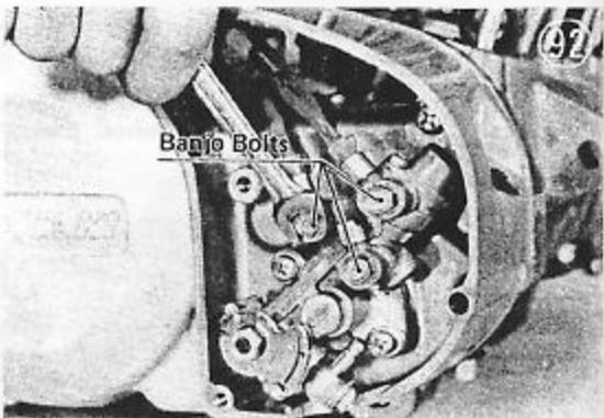
Drain the transmission oil. Remove the mounting screws and take off the right cover.
