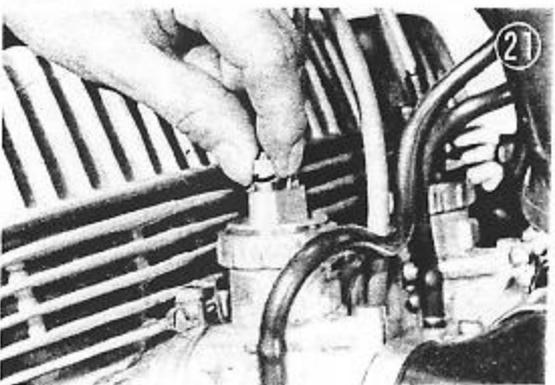
ii. S2, S3, KH400 : Back out each throttle stop screw until the throttle valves are in the fully closed position.
