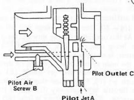
If the mixture is too rich, causes of this trouble might be clogging of the pilot air intake, or of the pilot jet air passage or air bleed opening. Possible causes of a lean mixture might be obstruction of the pilot jet or jet outlet. Other possible failures are included in the following table.
