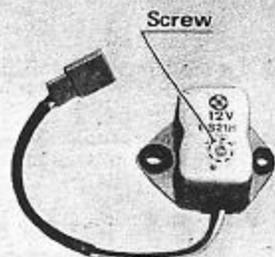
2. To avoid damage to the SVR, be sure the main switch is turned off before removing or replacing the unit.
