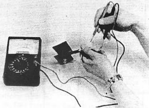
**NOTE:** In some multi-testers (ohmmeters) the batteries in the tester are reversed so that the current flow will appear to be the reverse of that shown in the table.
