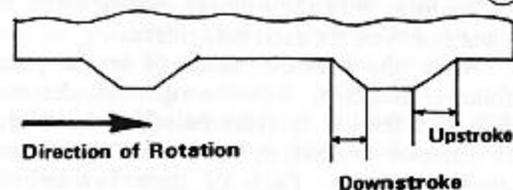
When the lowest part of the control cam is facing the plunger as shown in Fig. 174D, the plunger tip never touches the control cam and the cam on the plunger face can ride at point X from its highest to lowest point – the distance between the arrows. Accordingly, maximum plunger stroke occurs at maximum throttle opening.
