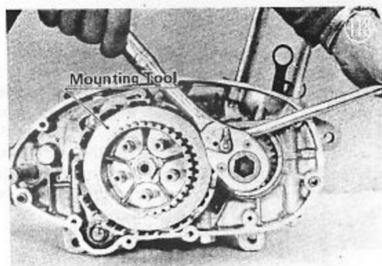
Remove the lock washer and primary gear.
