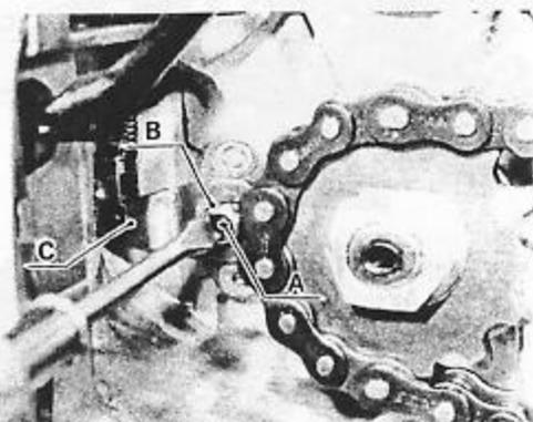
(2) Give the clutch hand lever play by loosening lock nut D and turning adjuster C, until the lever conforms with the measured position in the illustration.
