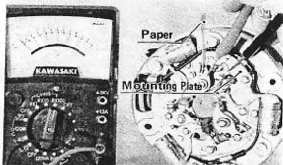
b. Check the contact points for wear or fouling. The points must be inspected periodically since they become worn after a long period of operation, and the slight sparking at each break gradually burns the surface.
