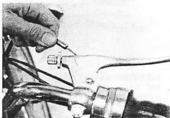
Loosen the front brake adjusting nut and pull the cable off the brake lever.
