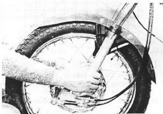
If the preceding inspection revealed play in the steering stem, the lock nut is not tightened sufficiently; if the steering was stiff, the lock nut is too tight and must be loosened.
