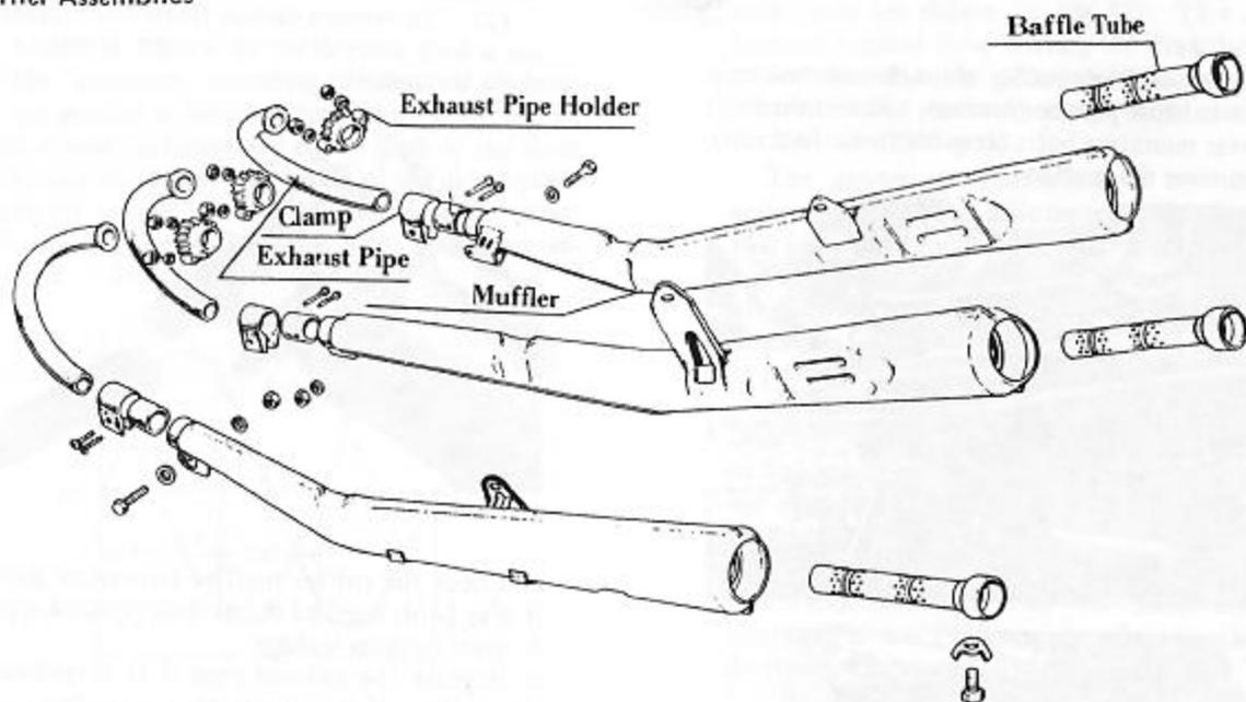
of the muffler. The exhaust gases from the engine are conducted to each muffler by the exhaust pipe. Inside the muffler the gas hits a baffle plate and enters the baffle tube through its many holes. When the gas strikes a baffle inside the tube, it exits into the muffler until
