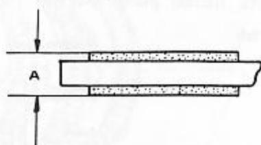
**Table 13 Friction Plate Thickness**
