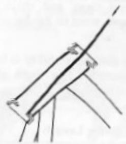
To remove the inner race from the steering stem, set a cold chisel to the point where the race and stem meet and hammer on the chisel lightly, moving it to different points so as to remove the race evenly. Be careful not to hammer too heavily as the stem will become misshapen.
