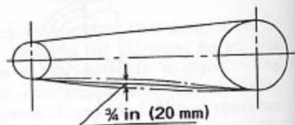
After adjustment, do not fail to retighten all the parts that were loosened. Also check rear brake adjustment.
