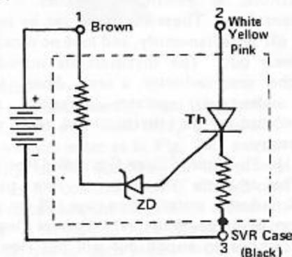
(4) Connect an additional 4 volts or so in series with the 12 volt battery, to make a total of over 16 volts, the breakdown voltage of the zener diode. Again check for current flow from ③ to ②. If current now flows, the regulator is operating correctly; if no current flows, either the zener diode or first thyristor is defective.
