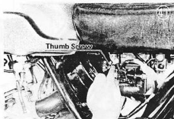
Pull air cleaner out through left side of frame. Take out two element mounting screws, remove element.
