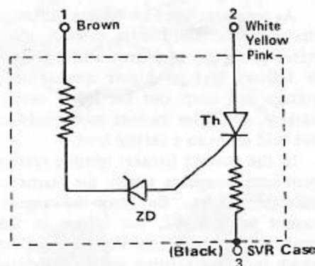
(3) Connect a 12 volt battery between ③ and ① with the negative lead to ③ and positive to ①, as shown in Fig. 387. Use an ohmmeter (tester) to see that current will not flow from ③ (-) to ①(+). If current flows, the zener diode is defective.
