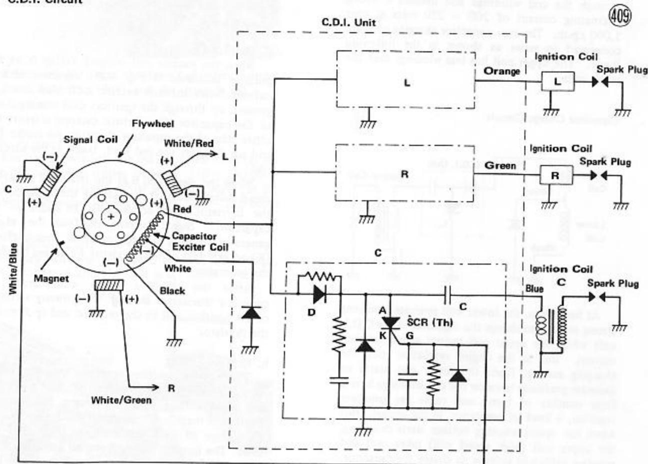
The chip of magnet is very small, but it has a strong magnetic flux. So when it cut through the coils instantaneously, the magnetic field in the coils changes so rapidly that a strong and sharp sine wave current is generated. This pulse current is sharp enough to trigger the thyristor in the C.D.I. unit without need of amplification. The three signal coils send signal current to ignite the spark plug in each cylinder at proper timing.
