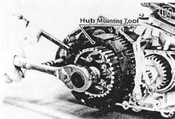
Take off the lock washer and flat washer. Remove the clutch hub, thrust washer and clutch housing from the drive shaft in that order.
