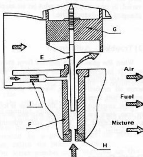
Among possible causes of faulty functioning would be obstruction or loose mounting of the main jet or needle jet, clogging of the air jet or needle jet, and jet needle wear.
